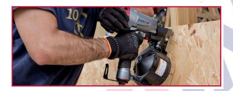
Paying close attention to the using habits of our customers; the EVERWIN siding nailer line up <u>SCN65C-ST</u> and <u>SCN65B-ST</u> have featured our patented precision nailing technology as well added depth adjustment features, this is key so fasteners aren't overdriven and may harm the surface material and lower the lifespan. It minimizes driver mark occurrences while maximizing line of sign in operation and ensures proper depth of nails.
