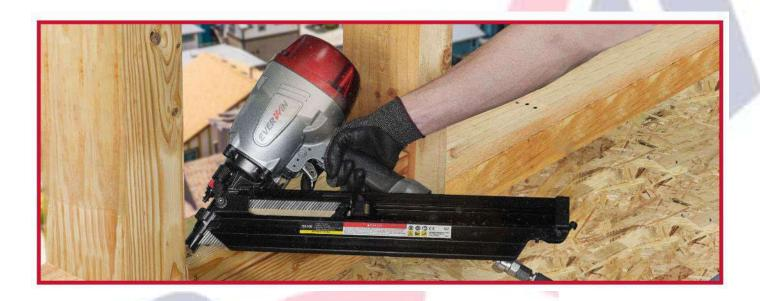
However, because of the high velocity, a framing nailer can leave marks on the work piece therefore they are less ideal for softwood siding or delicate lumber. This is not an issue in framing, if the nails are properly sunk into the timber. In fact, dept-adjustment is not required on framing nailers, such as the <u>FSN2283</u>. This simplifies the overall tool design and prolongs its lifespan.
